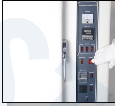
To set the parameter and control the testing
